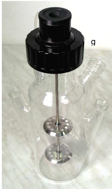
Fig. 10 The fermenter vessel with the head
