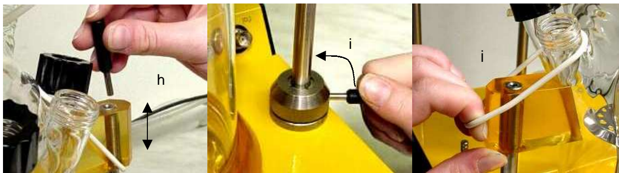
Fig. 11 Fixing the fermenter vessel onto the housing
