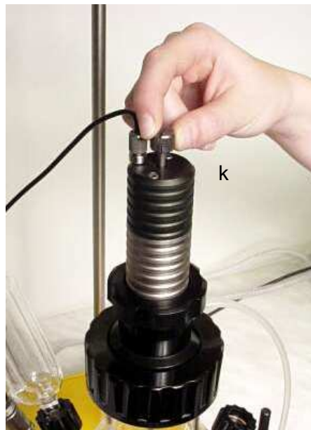
Fig. 16 Screwing of electromagnet
