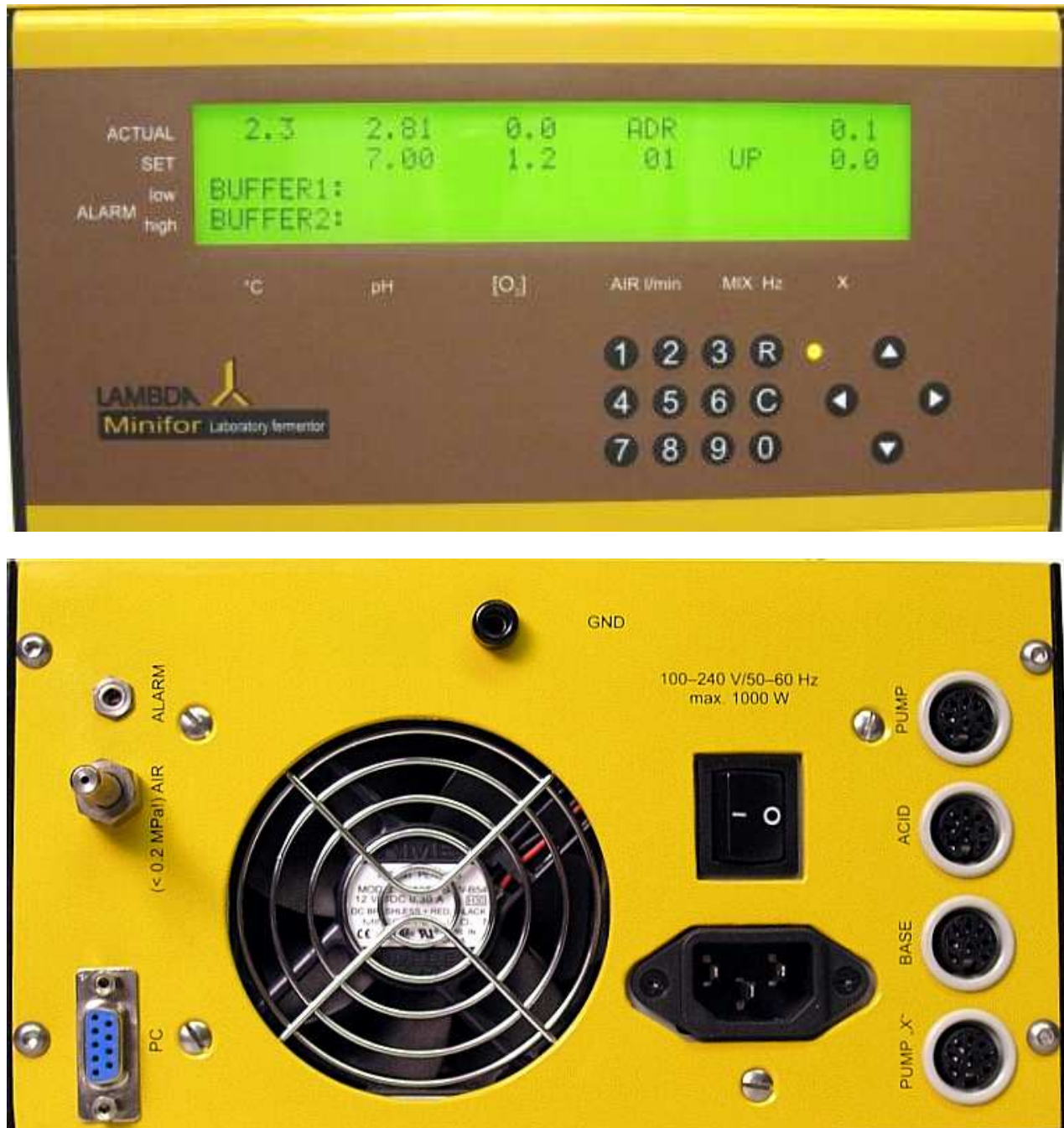
Fig. 1 Front side of the fermenter with control panel and back side of the fermenter
