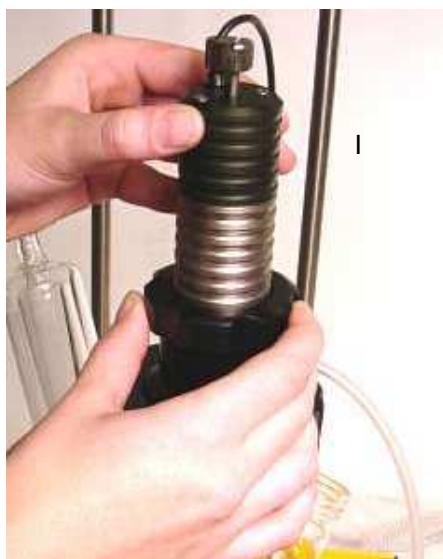
Fig. 17 Screwing of cap nut
