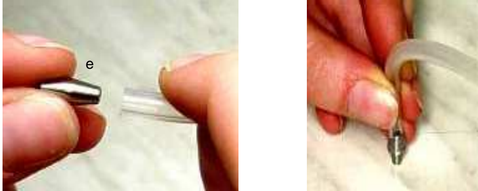
Fig. 4 A doubly conical insert is placed into the tube end
