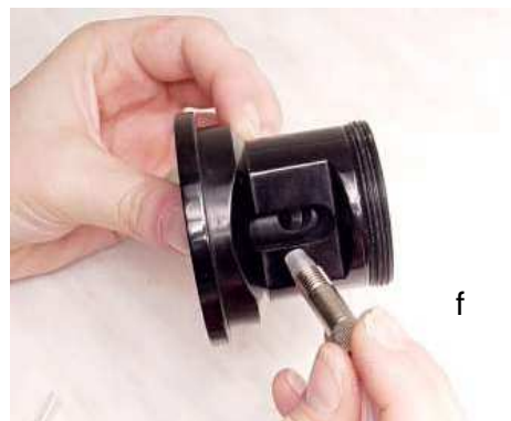
Fig. 5 Tube is screwed into the cock head
